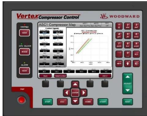
The Vertex controller is field configurable allowing users to configure/select the specific control algorithm required for the specific compressor loop and application. The control's special stage-to-stage and performance controller decoupling logic allows stable control during normal compressor operation as well as during plant upsets, minimizing process over or undershoot conditions.
