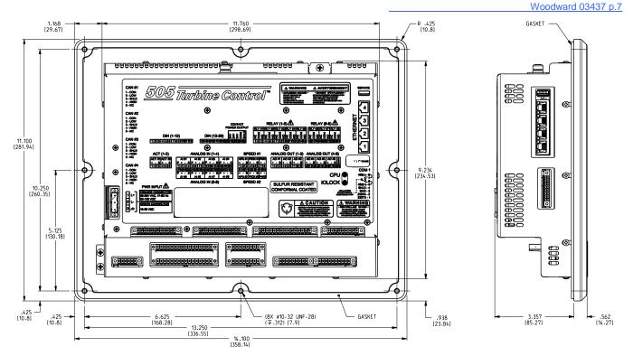
Figure 6. Vertex Control Package Dimensions
