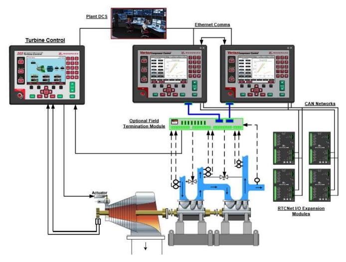
Figure 5. Typical Dual-Redundant Vertex Control Application
