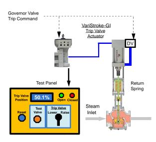
T&T Valve with new Hydraulic Actuator
