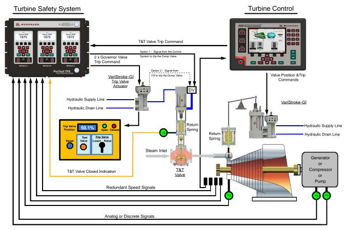
Figure 3. Typical VariStroke-GI Applications
