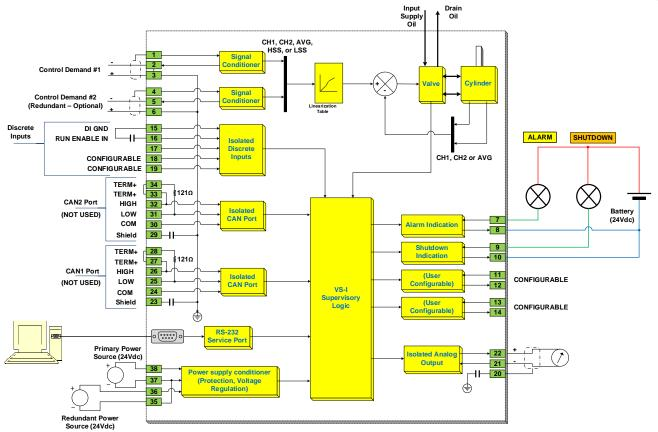
Figure 5. VariStroke-GI Interface
