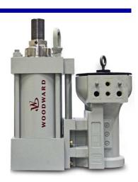
Single-acting actuators utilize an internal or external return spring to force the output shaft and connected valve to a safe closed position upon a shutdown event and have several advantages over double-acting actuators including fail-safe action as well as not requiring the use of expensive accumulators.
