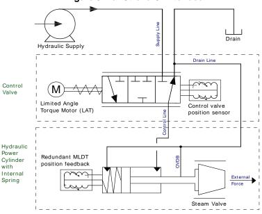
Figure 6. VariStroke-GI Hydraulic Diagram
