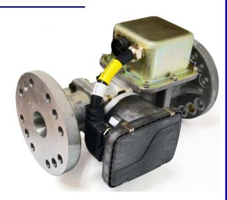
In general, a separate engine control system, like the E3 control, calculates the desired gas flow from the different engine and gas parameters. This desired gas flow is transmitted through a CAN link to the TecJet valve(s). The TecJet valve ensures that the desired gas flow is attained, automatically compensating for changes in gas pressure and gas temperature.
