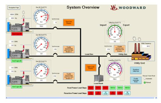
Students will learn the fundamentals of Speed Control, Speed Control Tuning, Power Generation, and Power Generation Control modes. This provides the student with a higher confidence level by developing practical skills and increased knowledge retention. The system module allows the student to start / stop engines, synchronize generators, add / subtract load, all through a realistic simulation model.
