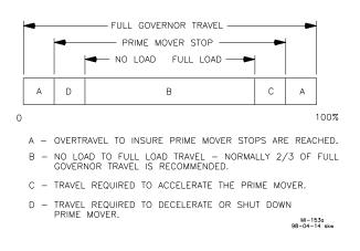
MAXIMUM WORK CAPACITY OVER FULL GOVERNOR TRAVEL OF 42\* IS \* . SEE ABOVE FOR RECOMMENDED GOVERNOR OUTPUT TRAVEL. IN SPECIAL APPLICATIONS MIN AND MAX PRIME MOVER STOPS MAY BE OUTSIDE THE GOVERNOR STOPS.
