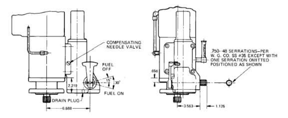
12 Ft-Lb Spring Loaded Rotary Power Servo
