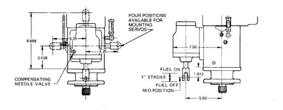
29/58 ft-lb Differential Power Servo (linear output)
