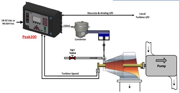
Figure 3. Typical Simple Peak200 Application
