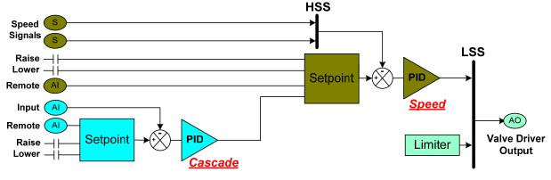
Figure 2. Basic Non-Ext/Adm Functional Control Diagram
