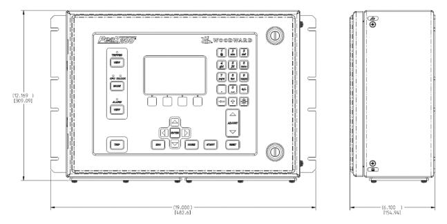
Figure 6. Peak200 Dimensions (Bulkhead Mount Models)
