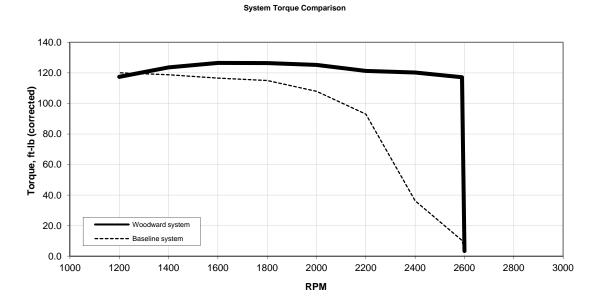
Torque vs RPM Curves (MI-04 compared to Baseline System)
