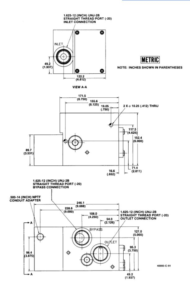
Outline Drawing of Liquid Shutoff Valve (Do not use for construction)
