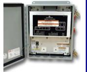
The controller system consists of a 16-bit CPU, sensor signal conditioning circuitry, a high-voltage power supply. and 20 (or optionally 24) outputs. The system can be configured from two cylinders to 20 (or 24) cylinders.
