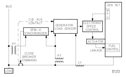
System Block Diagram Showing Optional SPM-A Synchronizer
