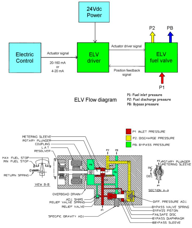
Schematic Diagram – ELV Liquid Fuel Valve
