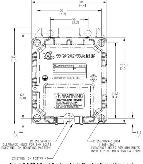
Figure 2. EDM-HD with 3-hole to 4-hole Mounting Bracket (top view) (Mounting Bracket only needed for installations with ICM 3-bolt mounting pattern)
