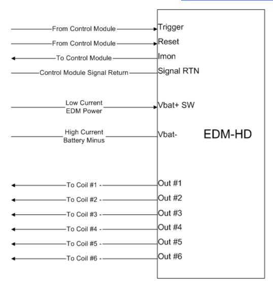
Figure 3. EDM-HD Six Cylinder System Connections
