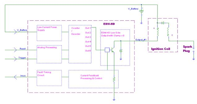
Figure 1. EDM-HD / Inductive Coil Simplified Block Diagram
