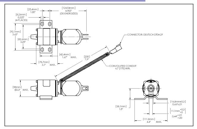
Figure 1. 0225 Actuator Dimensions (shown with Sheathed Leads)
