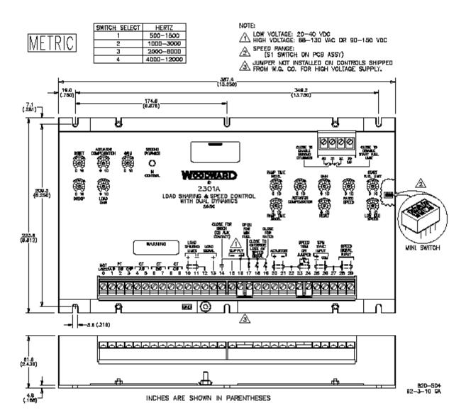
Outline Drawing of 2301A with Dual Dynamics (Do not use for construction)
