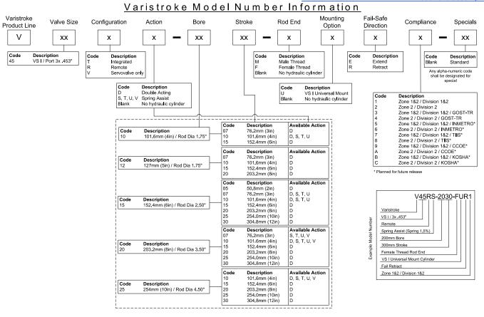
Figure 1. VariStroke-I Available Models / Ordering Number Encoder
