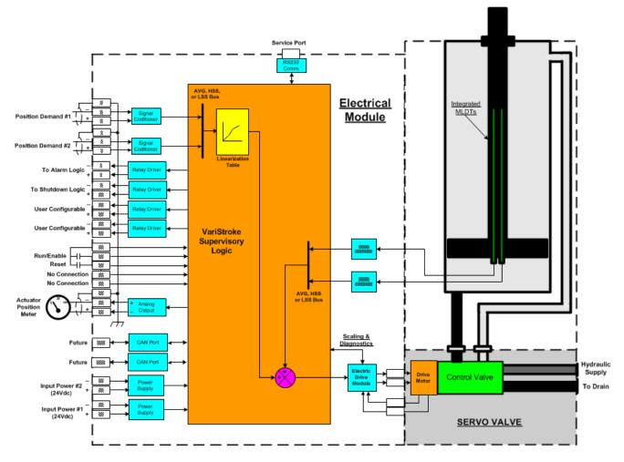
Figure 2. VariStroke-I Interface Schematic
